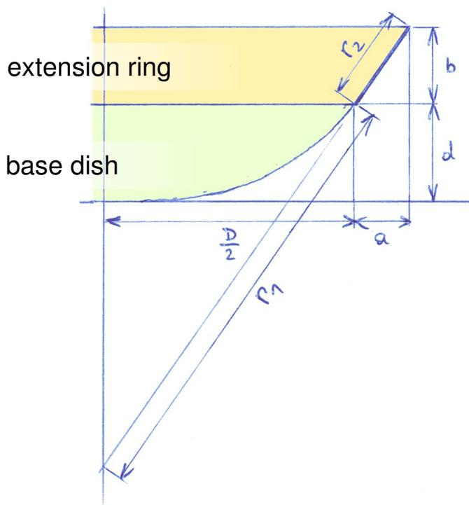
The extension ring is the surface of a section of a cone with the outer edge of  $(r_1 + r_2)$  and the radius  $(D/2 + a)$ .
